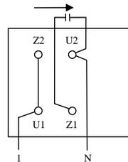
The arrows indicate the direction of rotation seen from the shaft side of the motor.
